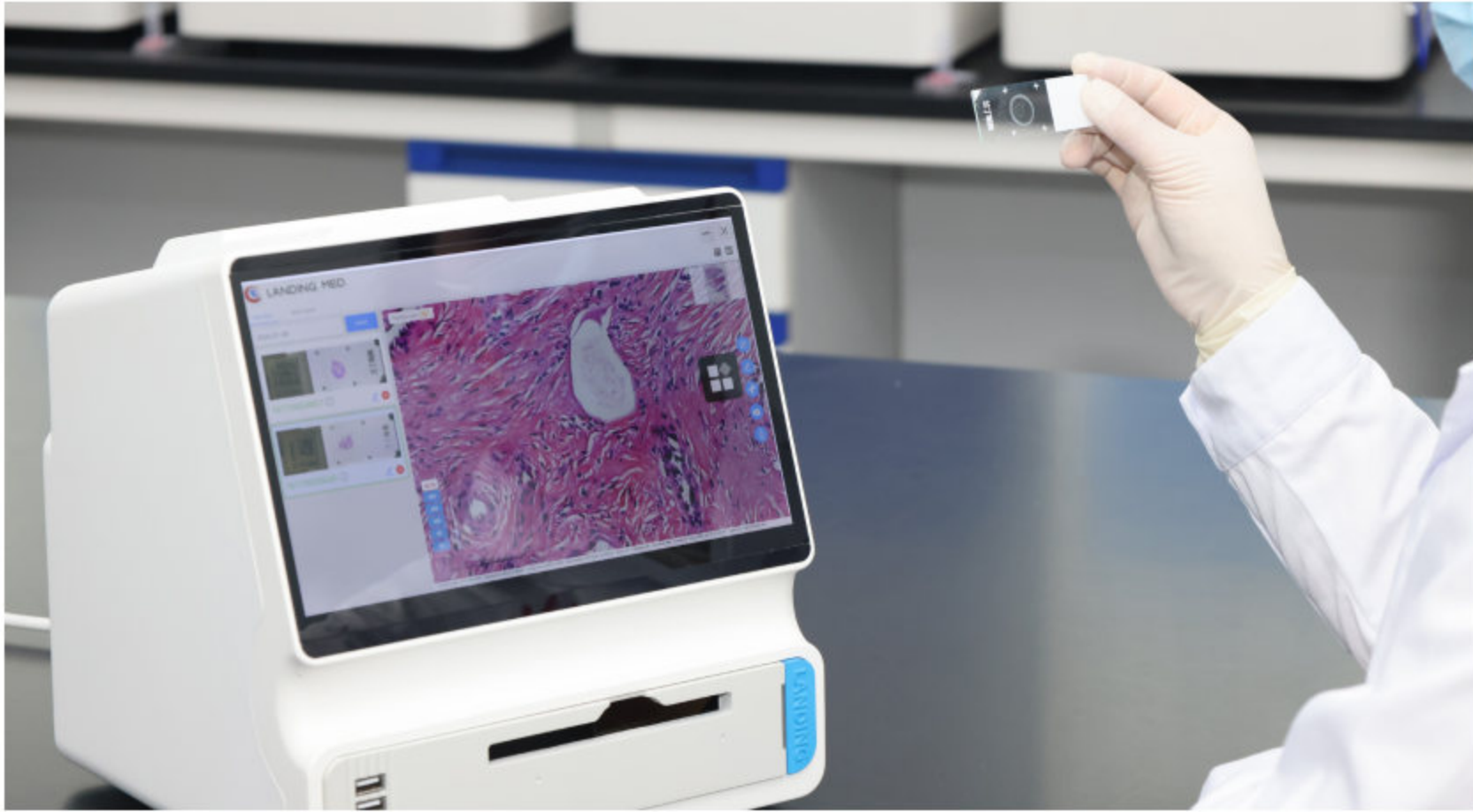
实验室人员使用显微图像扫描仪进行病理切片数字化扫描 A laboratory staff uses a microscopic image scanner to scan a pathological slide.
