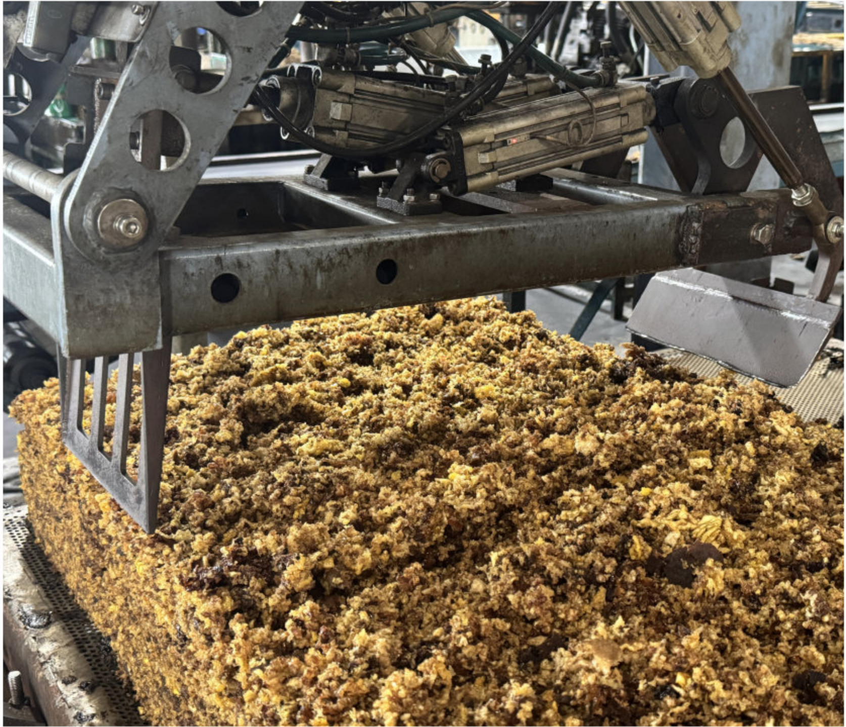
搭载 AI 算法的生产线自动将不规则橡胶半成品，完成工位间转移 An AI-powered production line automatically transfers semi-finished rubber blocks between workstations.
